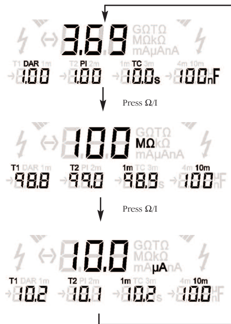
Figure 3 - The result of a dielectric discharge test (DD)
